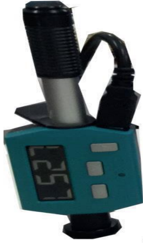
Figure 3 Equotip hardness tester used in the study
