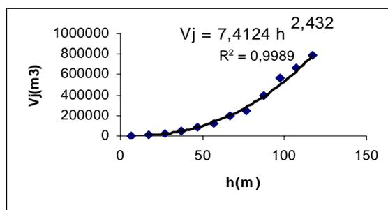
**Fig. 2.** Flotation tailing discharge volume out of the dump depending on the discharge column height
