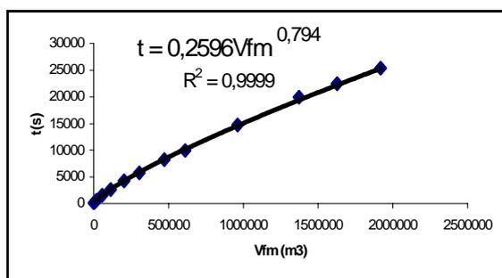
**Fig. 8.** Fluid mass discharge time through the abyss at the bottom of the dump “Valja Fundata”
