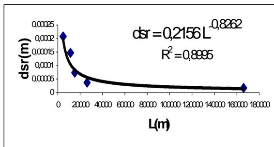
**Fig. 10.** Length of the flotation tailing particles transport depending on the average diameter
