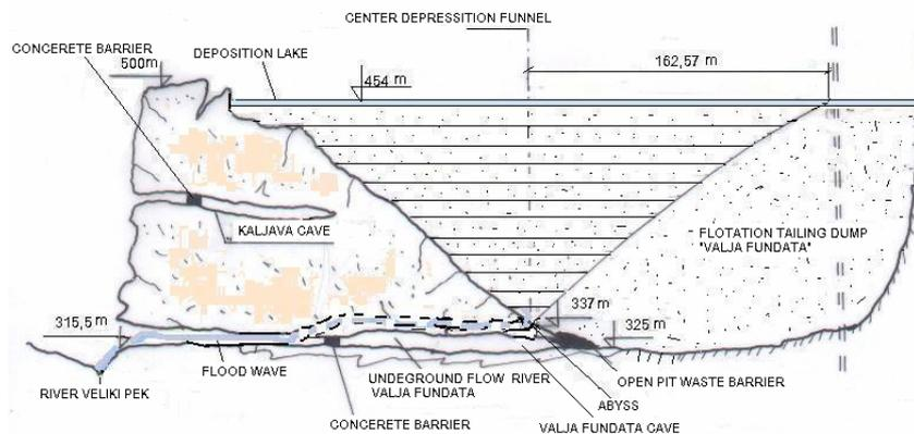
**Fig. 1.** Profile of the natural partition of the limestone massif with caves and the height of the precipitated tailing and clear water in the tailing dump in the moment of accident and the position of the depression funnel
