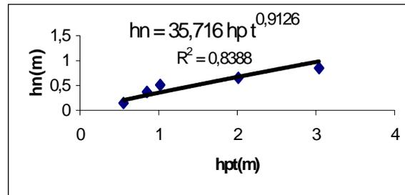
**Fig. 12.** Height of the flood wave on the flooded areas of the control points
