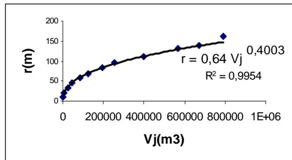
**Fig. 3.** Dependence of the depression funnel path line from the discharged tailing volume for each of the observed segments
