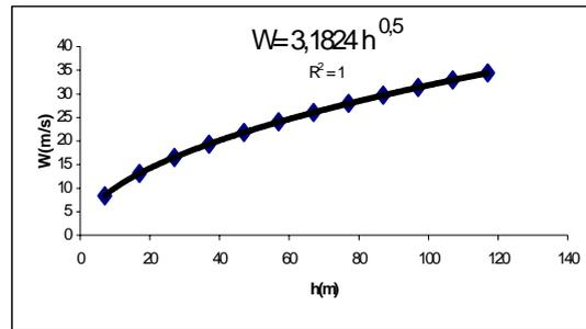
**Fig. 6.** Discharge speed of the fluid mass from the abyss depending on the discharge column height
