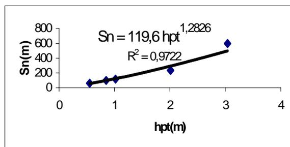
**Fig. 11.** Lateral width of the sediment on the flooded areas of the control points
