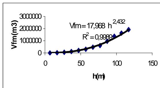
**Fig. 5.** Fluid mass discharge depending on change of the discharge column height
