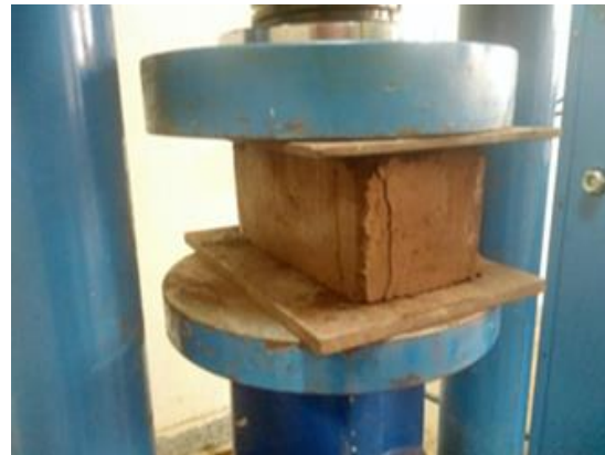
Figure 6. Compressive strength test of Brick Samples
