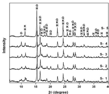
**Figure 2.** XRD pattern of +150  $\mu\text{m}$  (S-1), +125  $\mu\text{m}$  (S-2), +106  $\mu\text{m}$  (S-3), +90  $\mu\text{m}$  (S-4) and +75  $\mu\text{m}$  (S-5) sieve fractions. H=Hematite, G=Goethite, K=kaolinite.
