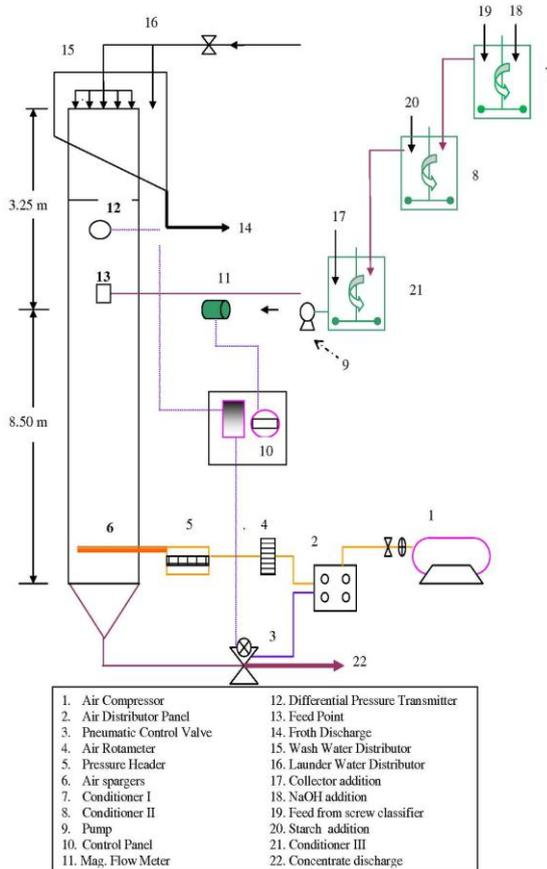
**Figure 1.** Schematic diagram of the 0.5 m dia flotation column
