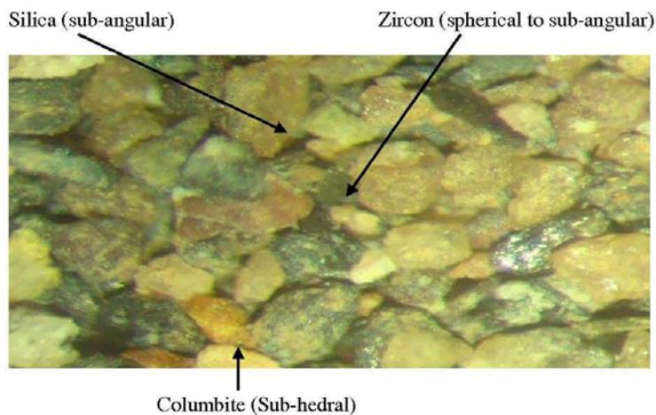
**Figure 2b.** Microscopic view of the shapes of the compositions of the tailings 100×
