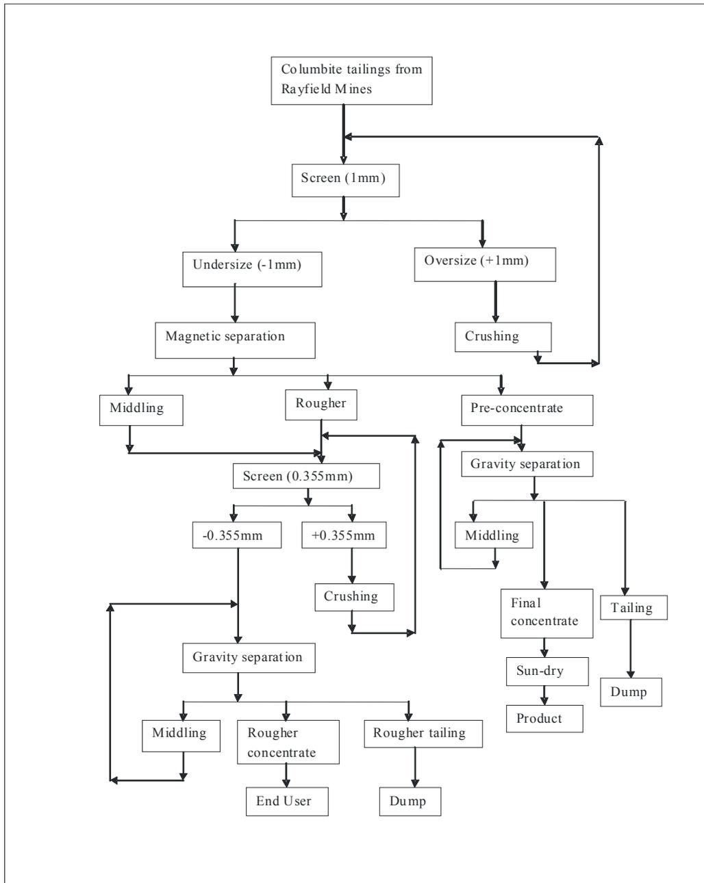
**Figure 1.** The wet processing flowsheet
