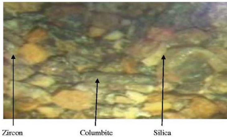
**Figure 2c.** Microscopic view showing the colours of the composition of the tailings 100×
