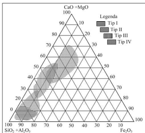
**Figure 1.** The three-component diagram SiO<sub>2</sub>+Al<sub>2</sub>O<sub>3</sub>, Cao+MgO and Fe<sub>2</sub>O<sub>3</sub> of fly ash**Explanation:**
